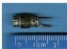
**FIGURE 1.7** A transistor, which replaced the vacuum tube
